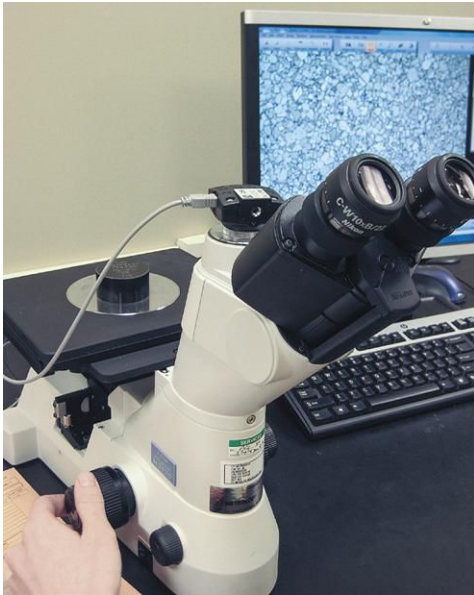
Grain-size evaluation of Inconel 718 at 100X magnification using a light optical microscope.
