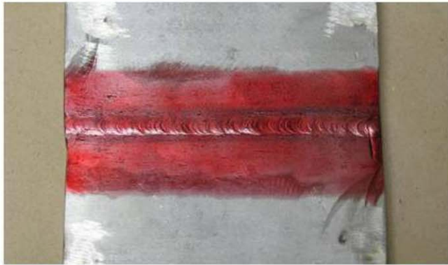
Both the visible and fluorescent dye penetrants can be applied to the test sample by spraying, brushing or immersing the part in a penetrant bath. Source: Laboratory Testing Inc.
