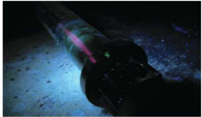
When working with fluorescent penetrants, indications must be viewed under darkened conditions with a high-intensity UV lamp or black light. Source: Laboratory Testing Inc.
