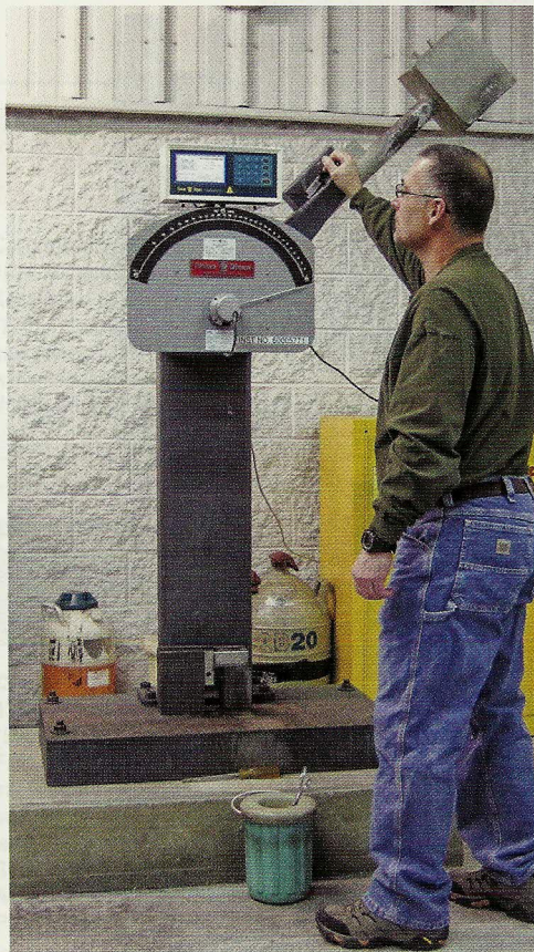
A technician conducts Charpy impact testing.
