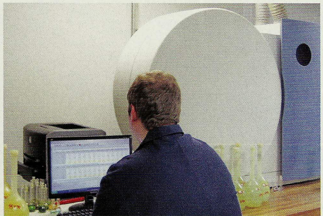
ICP-AES analysis is an instrumented wet chemistry method.
