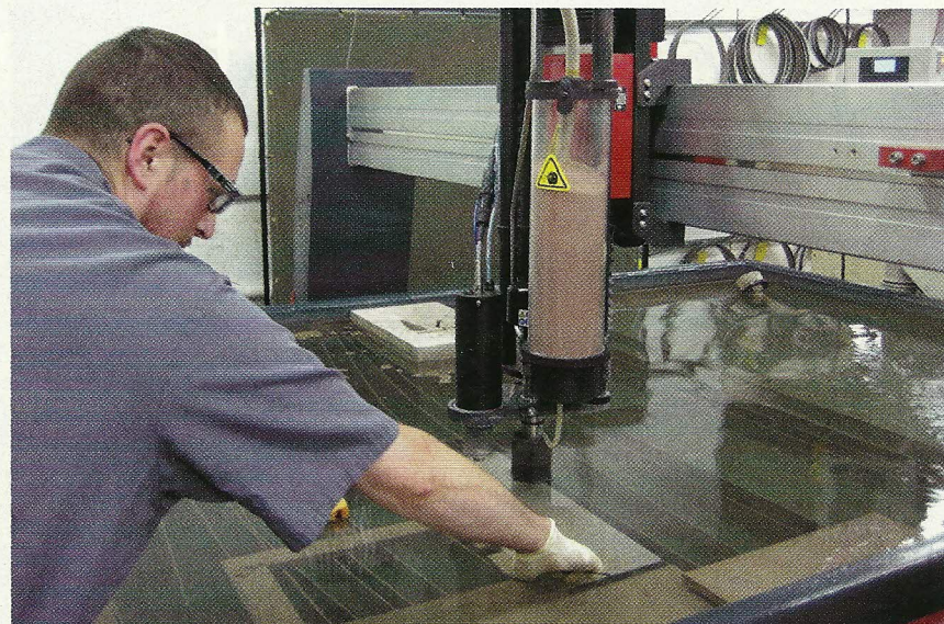
Cass sets up a 1/8-inch-thick stainless steel sheet from which to cut near net shape specimens on the MaxiM 1515 abrasive waterjet system.
