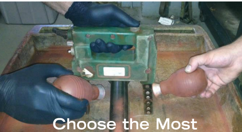
This is a visible dry powder MPI using a portable yoke. Source: Laboratory Testing Inc.
