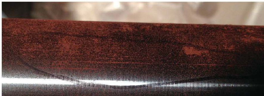
These are linear indications observed using visible dry powder and direct current. Source: Laboratory Testing Inc.
