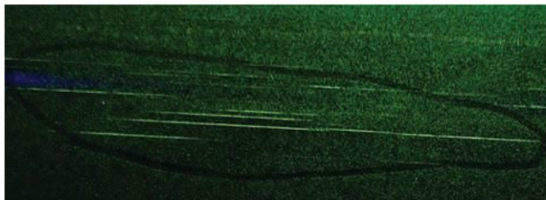
Here are linear indications observed using fluorescent wet particles. The multiple linear indications believed to be inclusions/stringers in the machined areas were even more pronounced and much more populous than observed by the previous visible dry powder inspection. Source: Laboratory Testing Inc.
